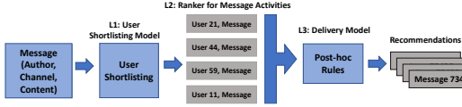
Figure 2: The current Production System deploys a three layer architecture with layers– L1: user weaning, L2: message classification and L3: personalized delivery model. Our model is relevant for the L2 layer and is evaluated against the production-grade models for the L2 layer.
